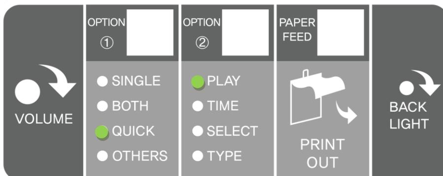
While pressing the [PAPER FEED], Press the [OPTION 1] button to select the test mode.
