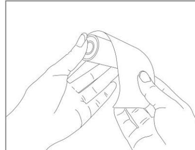
2. Put the paper in the paper tray and align the paper in the middle of the rollers.
