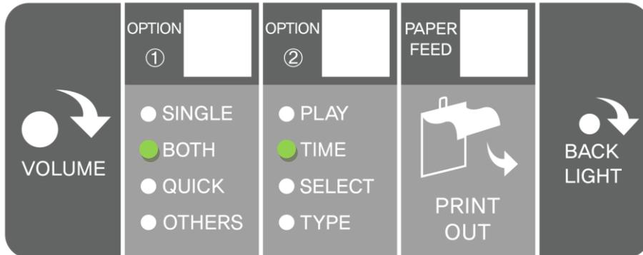
While pressing the [PAPER FEED] button, Press the [OPTION 2] button to [TIME] and current time is printed out from thermal printer.
